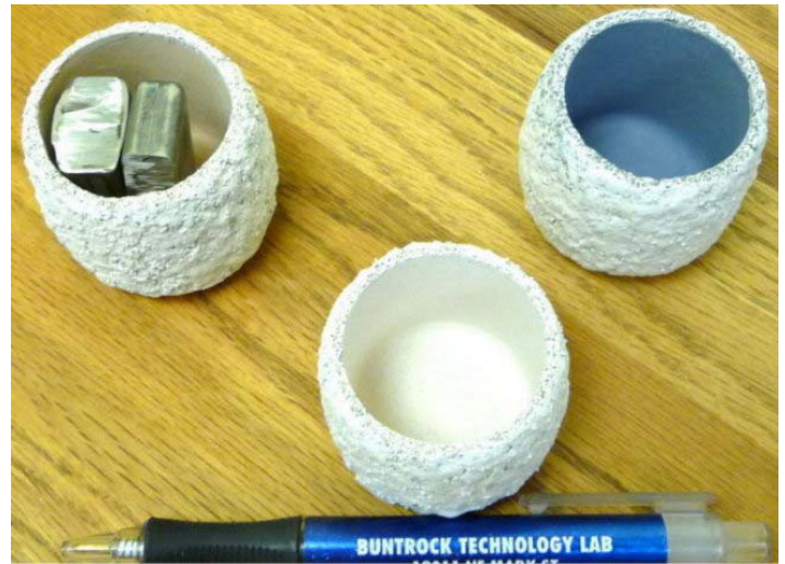
Picture 2. Crucibles made of various inner materials to be evaluated as zircon substitutes.
