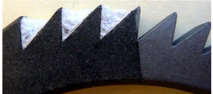
Picture 1. Casting of 17-4 SS at 2900F using Cerabeads 60 Stucco
