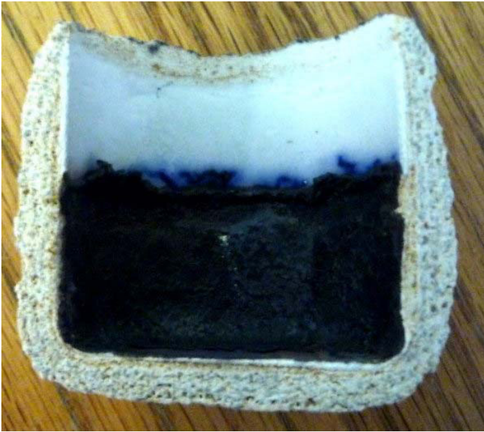
Picture 4. Tabular Alumina Prime layers with Wing Beads Stucco
