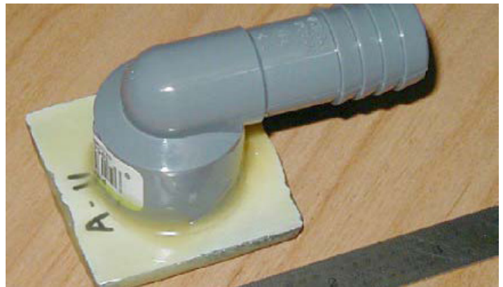
Figure 3. Plastic fitting sealed onto face of shell sample.
