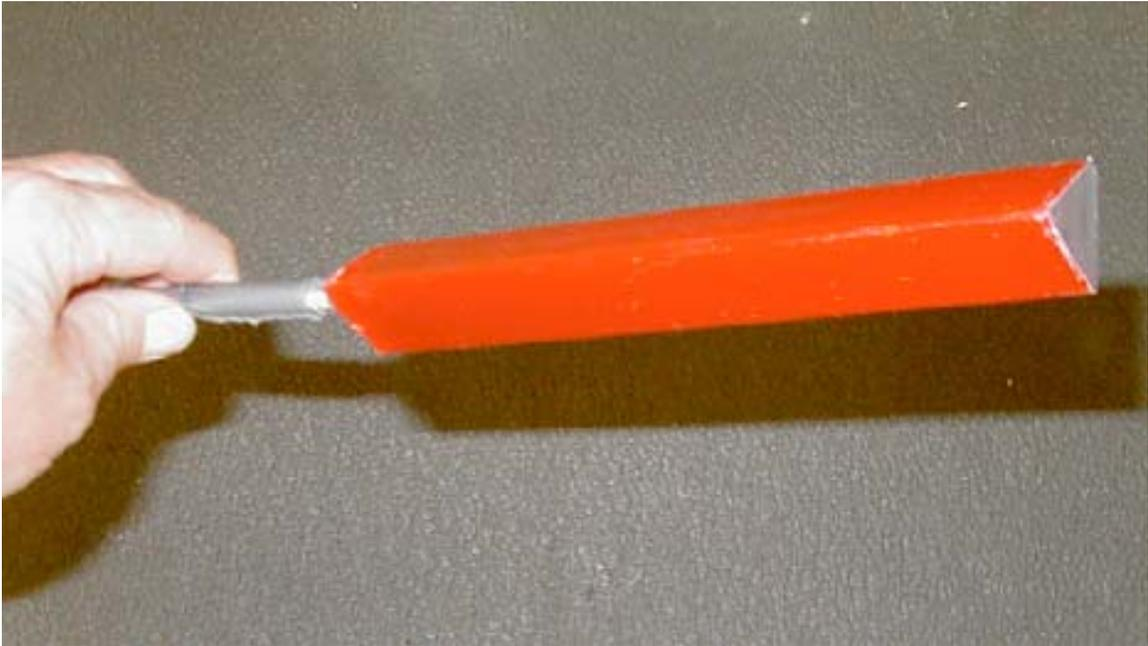
**Figure 2. Sectioned and dewaxed Shell Build specimens ready to be measured.**
