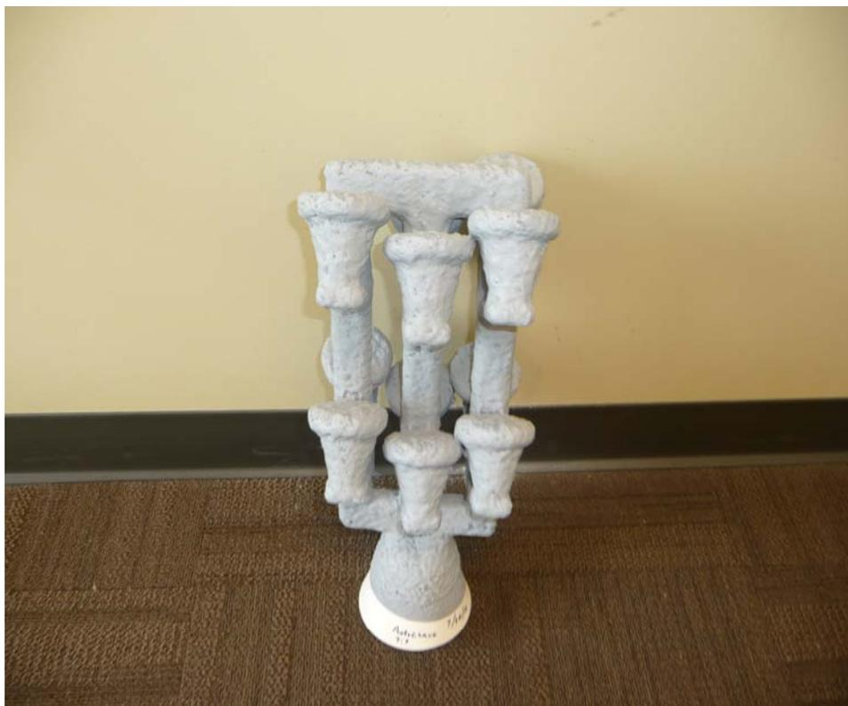
Figure 6 – Fibercoat 1109 shell after autoclave dewax.
