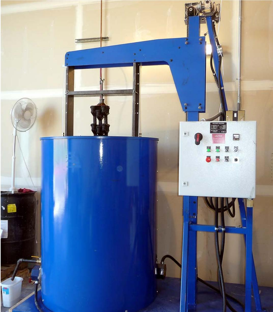
Figure 2 – Prototype directional dewax, hot oil dewax equipment
