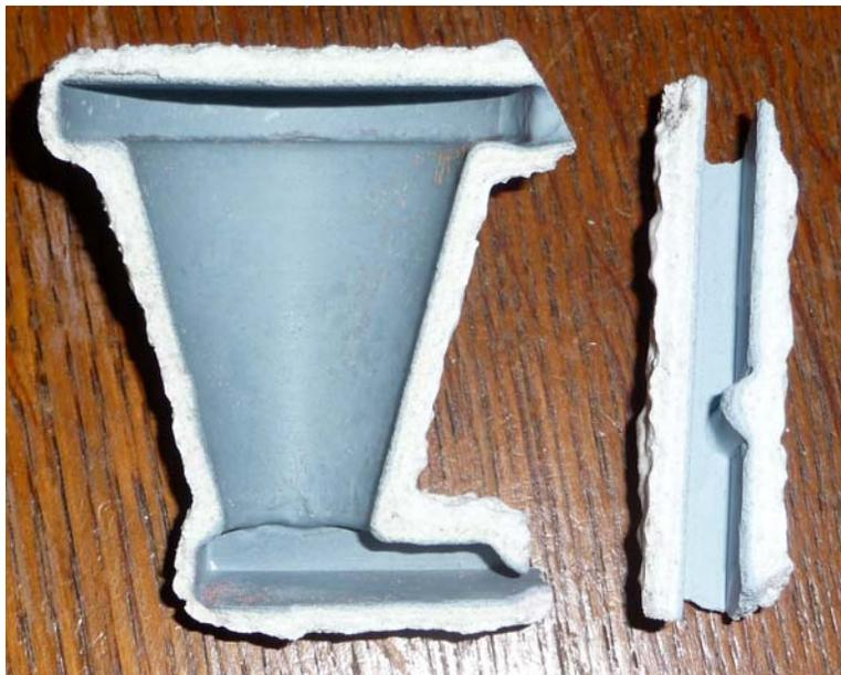
Figure 9 – Fused silica backup shell with 2 backup dips and restriction in gating.
