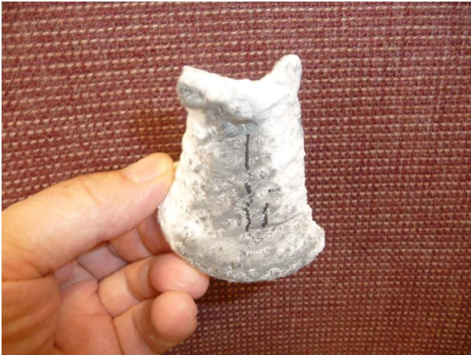
Figure 7 – Through wall crack on Fibercoat 1109 shell after flash fire dewax.
