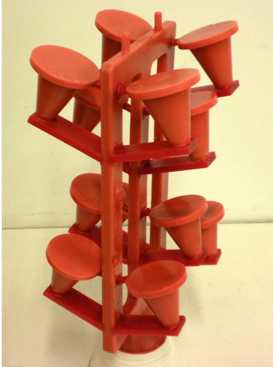
Figure 3 – Crack prone wax assembly 18” tall.
