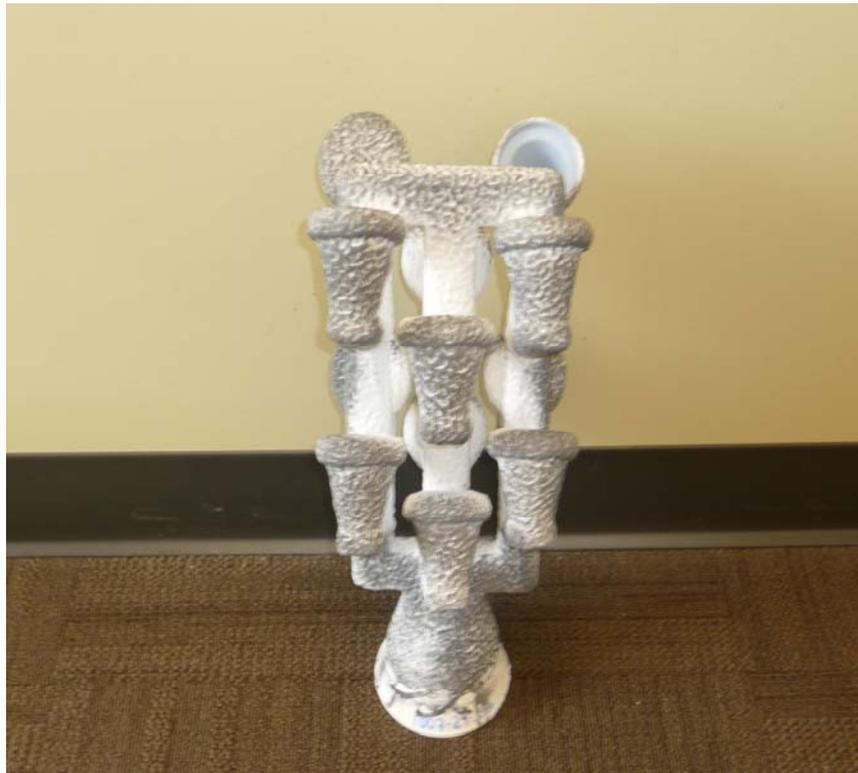
Figure 5 – Fused Silica shell after flash fire dewax.
