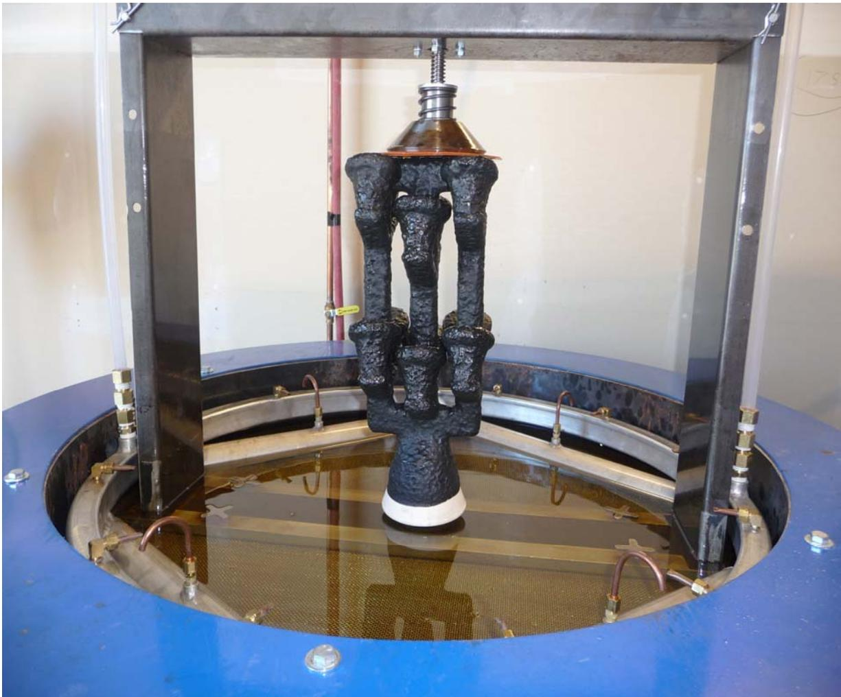
Figure 4 – Fibercoat 1109 shell after directional hot oil wax removal.
