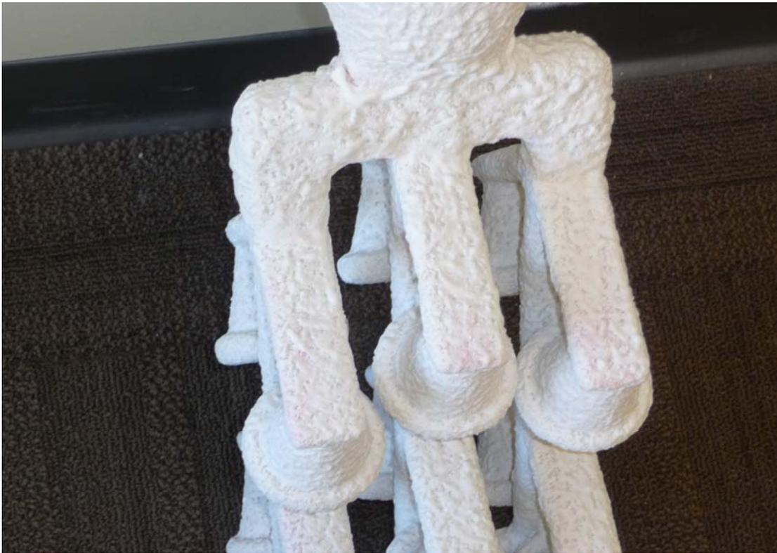
Figure 11 – Fused silica thin shell, autoclaved, restricted gating. All 12 gates cracked. Red wax bleeding through shell because of cracks.
