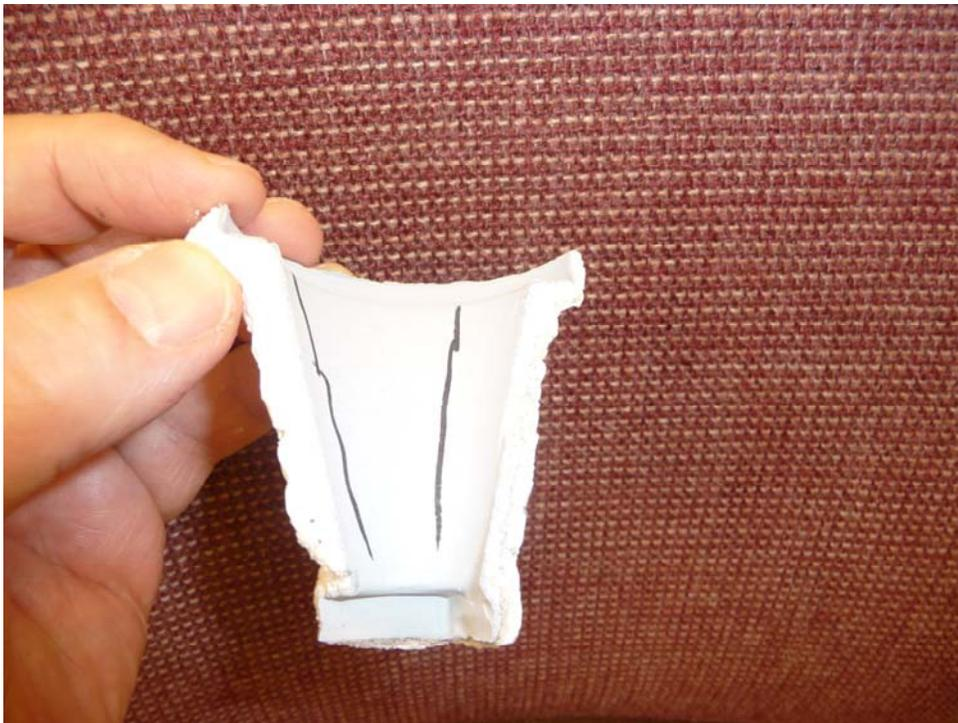
Figure 8 – Interior cracks on prime coat of Fibercoat 1109 after autoclave.
