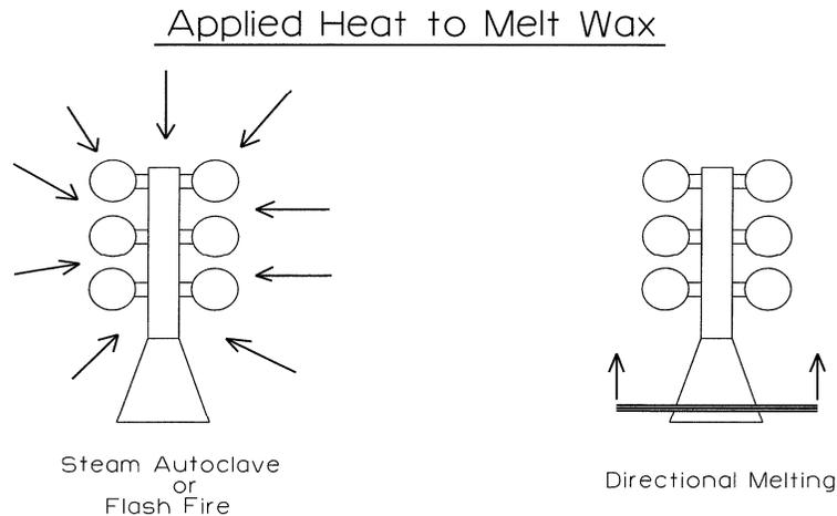
Figure 1. Comparison of traditional dewax and directional wax removal.
