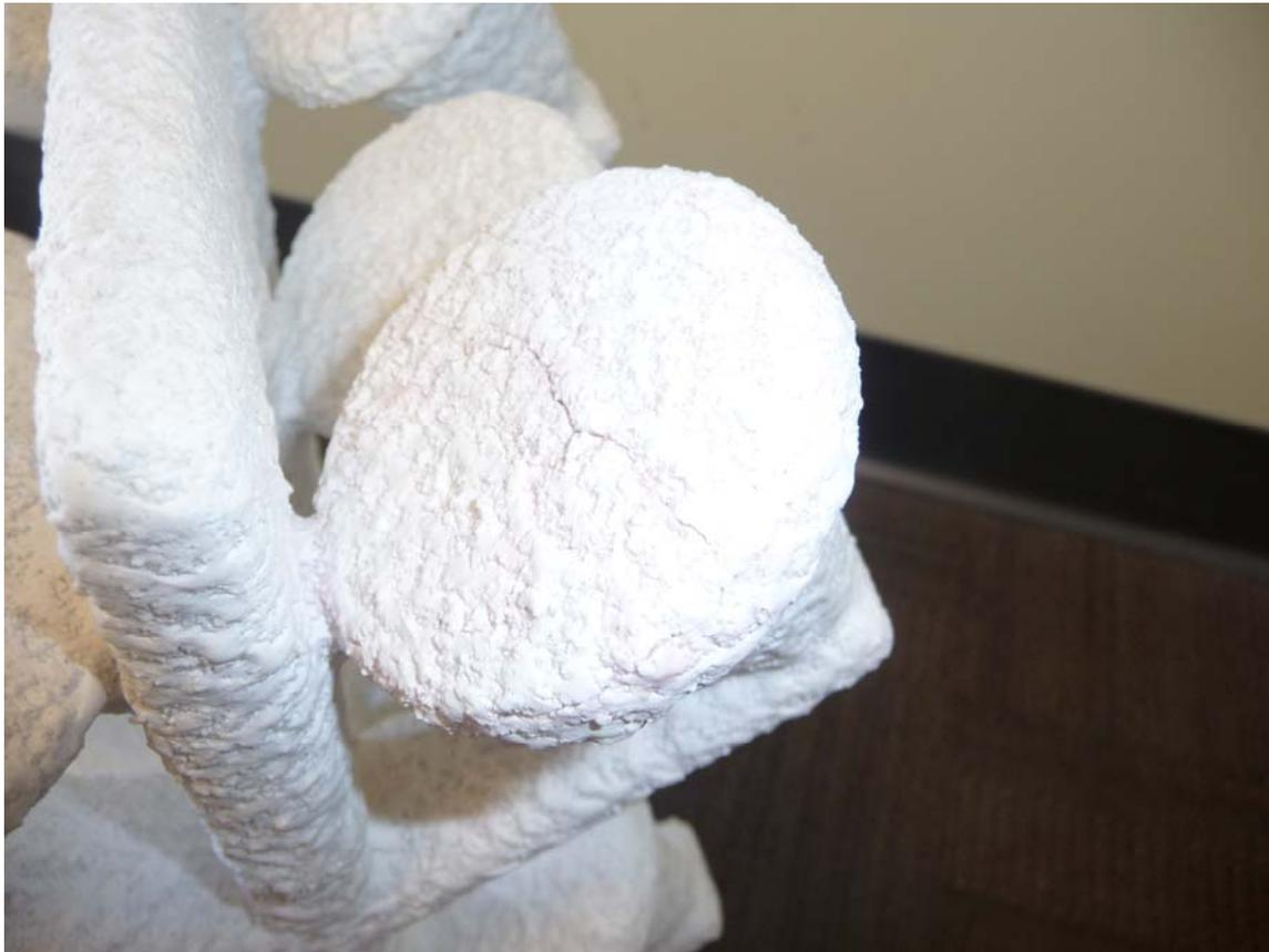
Figure 10 – Severely cracked fused silica thin shell, autoclave dewax, restricted gate.
