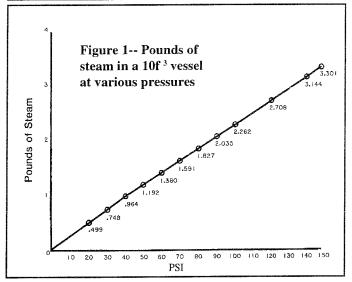
containing 19,125 BTUs (British Thermal Units), to fill the 79.3 cubic feet (f³) vessel to a pressure of 90 pounds per square inch (PSI).
