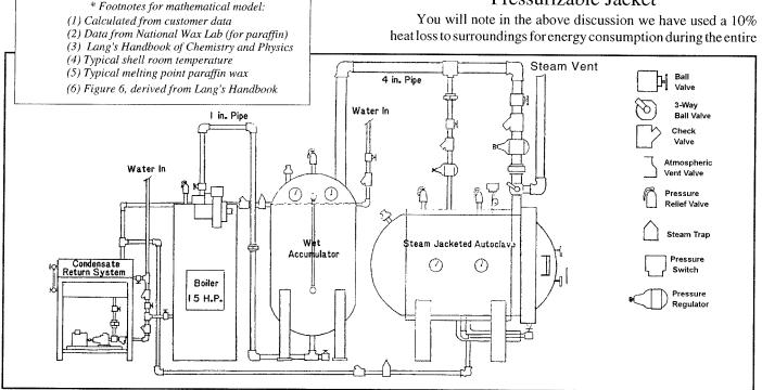
cycle. For our "instantaneous BTU work demand" we have again applied equation two, but then allowed no such energy loss. This is probably acceptable due to the instantaneous nature of our surge pressurization, but it also presumes the use of preheated and pressurizable jacket surrounding the autoclave. With sufficiently preheated vessel sidewalls, their BTU energy absorption during pressurization can be considered nil.
