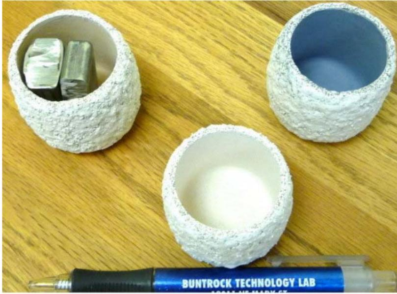
Picture 2. Crucibles made of various inner materials to be evaluated as zircon substitutes.
