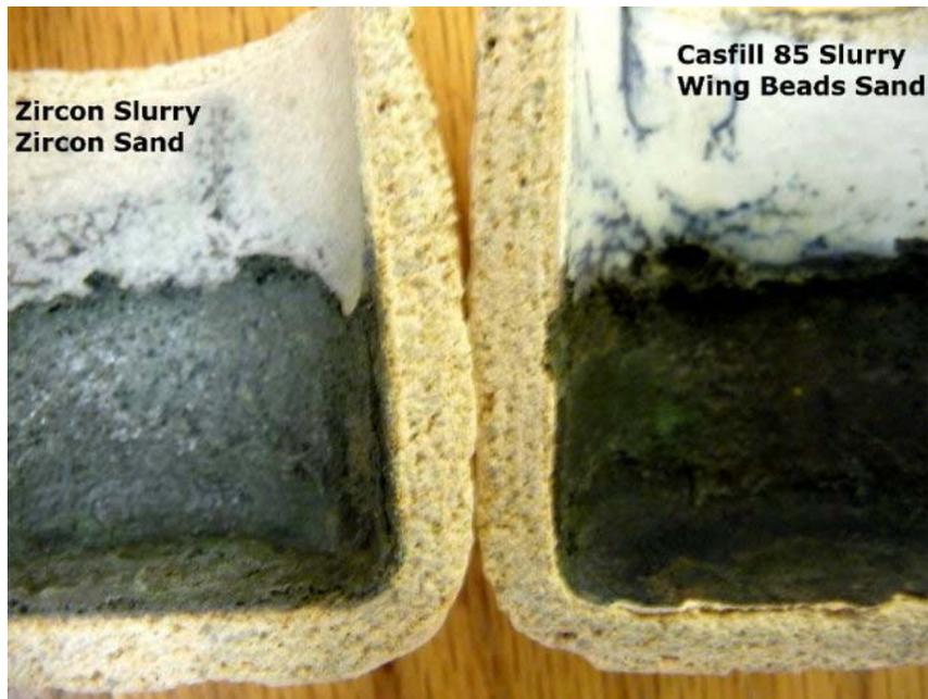
Picture 3. Comparison of zircon and Casfill 85 inner layers
