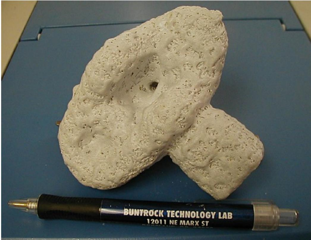
**Figure 2. Dewaxed Part – Coated Stucco One Shift Shell.**
