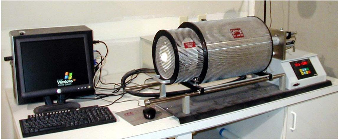
*Figure 1. Orton Dilatometer 1600C*
