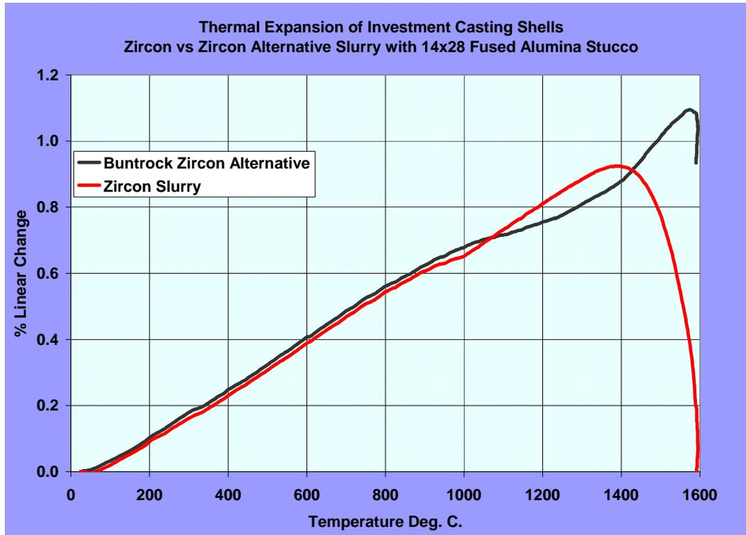
*Figure 7. Thermal Expansion of a typical Zircon Slurry, Alumina Stucco DS shell. A Zircon Flour Alternative is also shown.*
