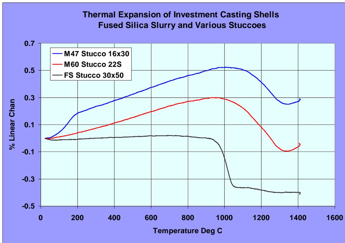
**Figure 3. Thermal Expansion of Fused Silica Slurry with Fused Silica, Mulgrain 47, and Mulgrain 60 Stucco.**
