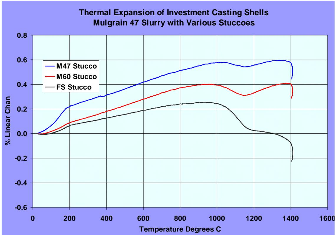
*Figure 5. Thermal Expansion of Shells made with Mulgrain 47 Slurry and Various Stuccoes*
