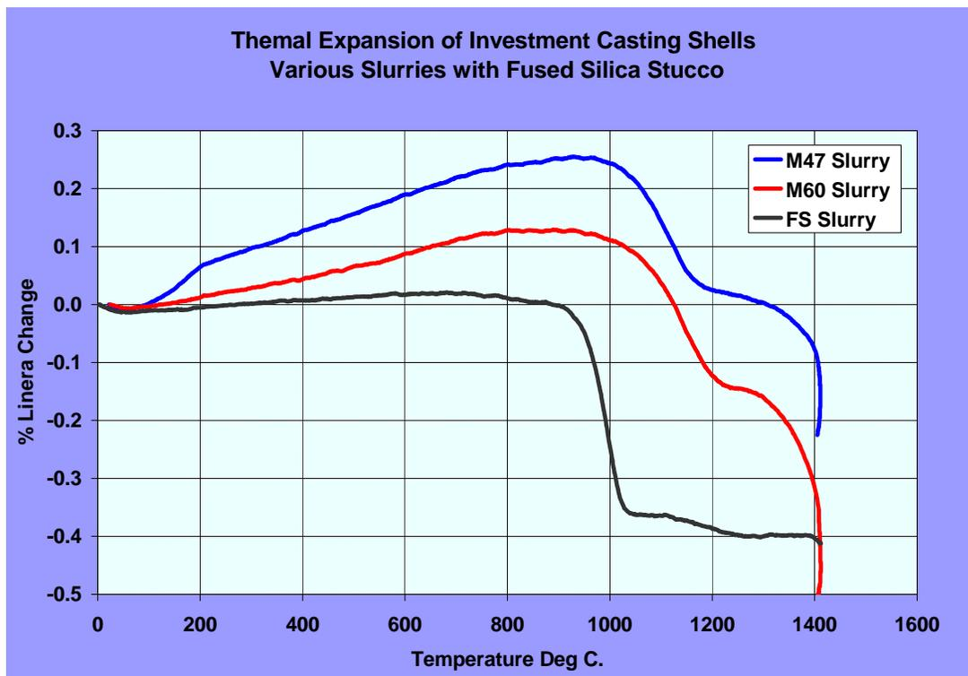
*Figure 4. Thermal Expansion of Shells made with Different Slurries all using Fused Silica Stucco*
