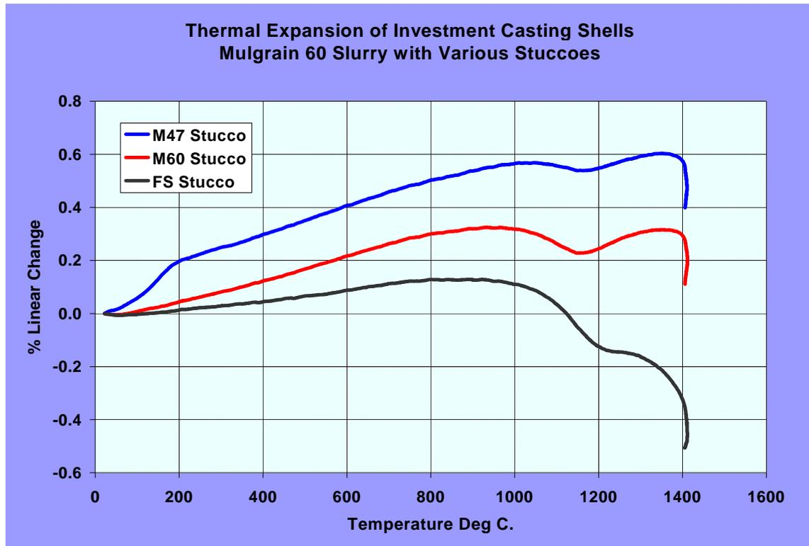
*Figure 6. Thermal Expansion of Shells made with Mulgrain 60 slurry and Various Stuccoes*
