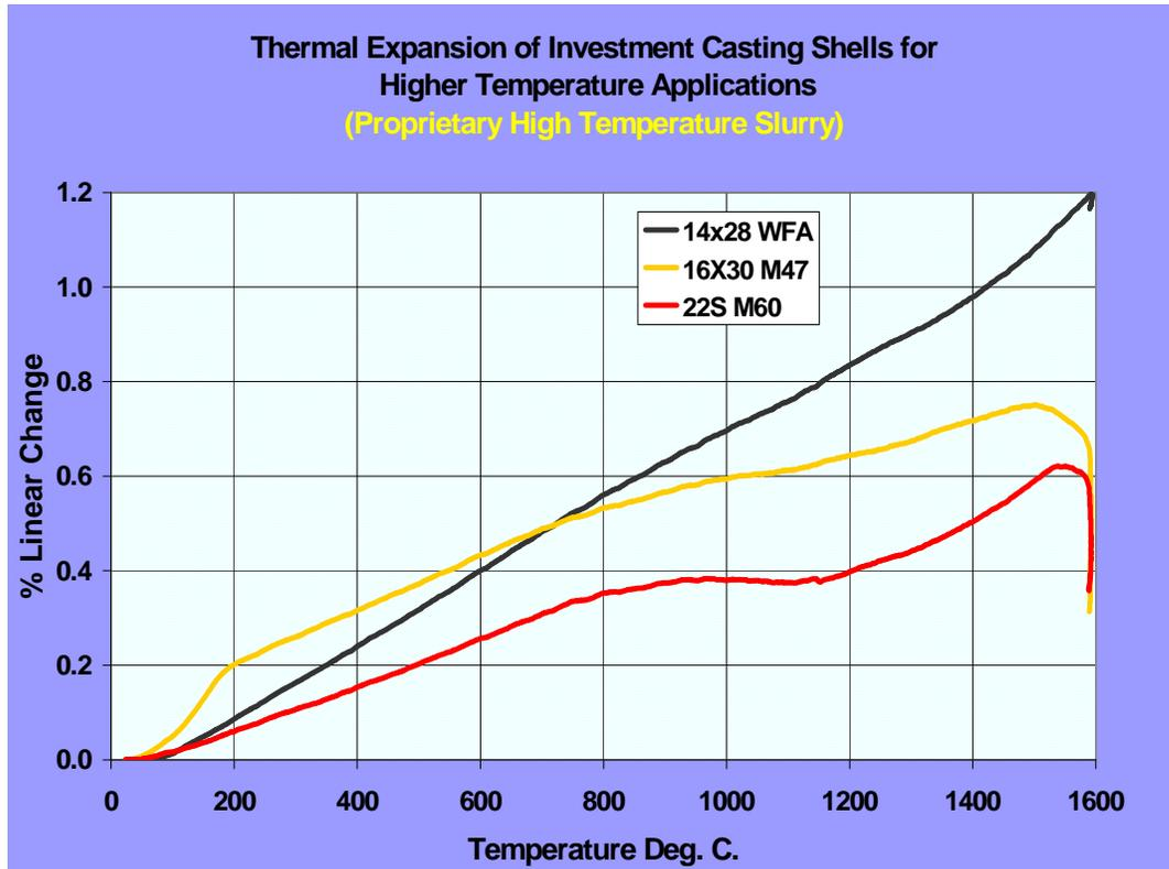
*Figure 8. Thermal Expansion of Very High Temperature Shell with Various Stuccoes*
