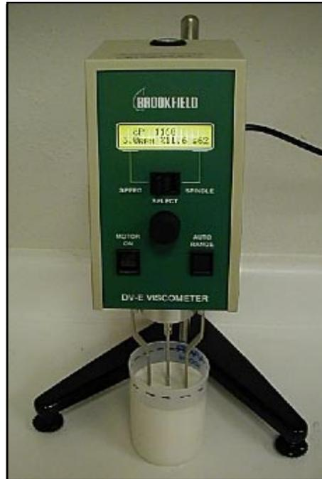
Figure 3. Brookfield Viscometer
