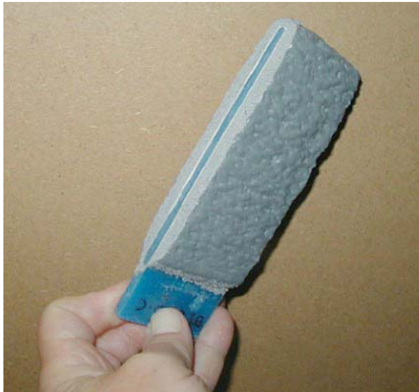
Figure 2. Shell dipped on wax and edges ground for removal from wax.
