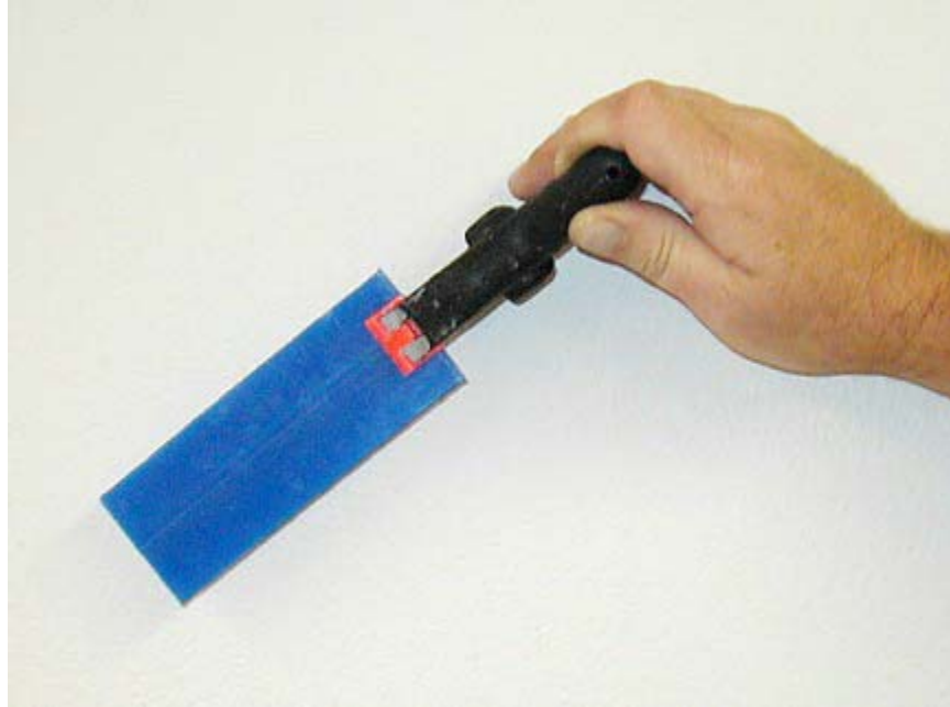
Figure 2. Shell dipped on wax and edges ground for removal from wax.
